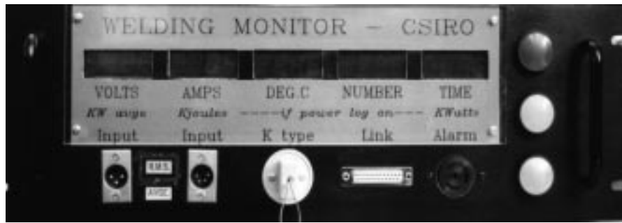
Figure 4-3 Welding Data Monitor (WDM)
